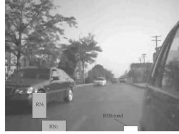
Fig. 8 The check regions for closing vehicle detection.
