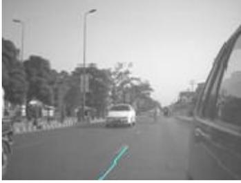
Fig. 6 Detected inner boundary of lane.
