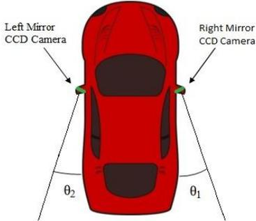
Fig. 1 CCD cameras mounted on the side mirrors of vehicle
