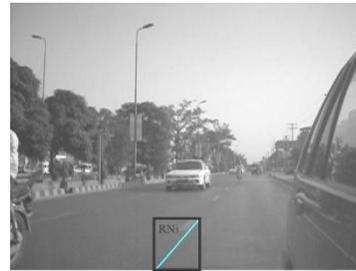
Fig. 10 ROI for the detection of true lane marking candidate.
