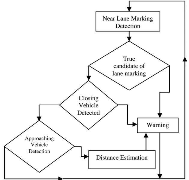
Fig. 4 The flow chart of lane marking and vehicle detection.
